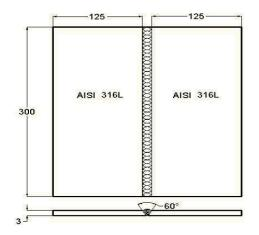
Fig. 1. The welded plate of 316L SS.
