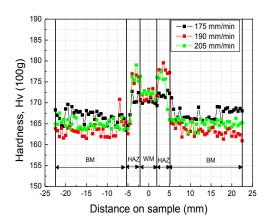
Fig. 3. Vickers micro-hardness result for different welding speed conditions.
