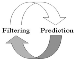
Fig. 9. Continuous loop of Kalman filter algorithm
