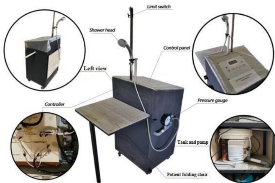
Figure 3. Automatic therapeutic shower prototype
