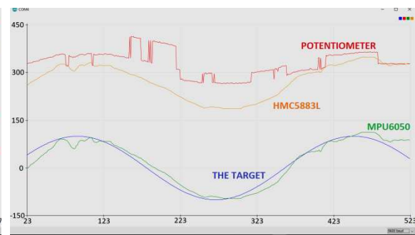
Figure 9. The sine wave target and performance of the three sensors at the steering position
