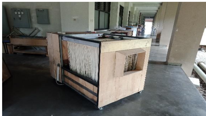
Gambar 2.1 Unit air cooler
