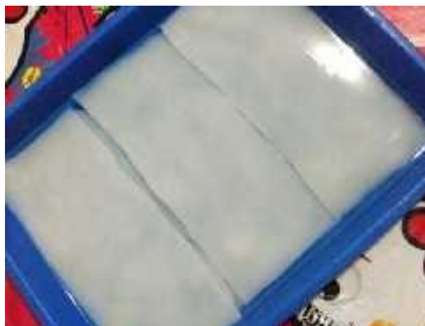
FIGURE 1. The bacterial cellulose film initiated by Acetobacter xylinum incubated at 30^\circ\text{C} for 7 days
