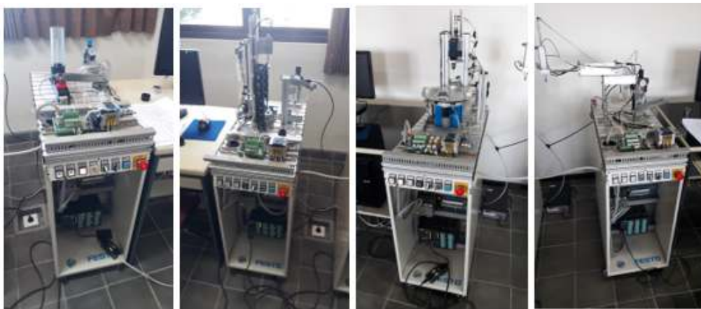
Figure 4. Modular Production System (MPS), a=Distribution Station, b=Testing Station, c=Processing Station, d=Handling Station.
