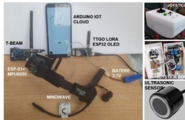
Figure 5. Components or devices used in the electric wheelchair control system, including Arduino IoT Cloud
