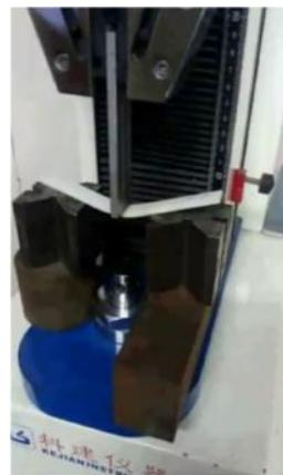
Gambar 9. Proses bending test
