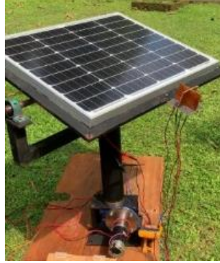
FIGURE 6. The physical form of LDR, DC motor, and solar panel.
