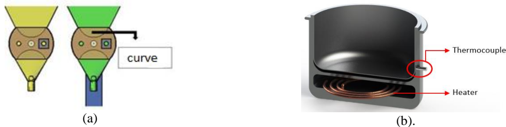
FIGURE 2. (a). Rotary vane feeder design with 2 curves and photodiode, (b). The design of a cooking kettle equipped with a thermocouple and heater
