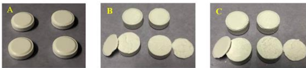
Figure 1. The organoleptic of paracetamol tablet resulted from Formula 1 (A) first compression tablet (B) first recompression tablet (C) second recompressed tablet
