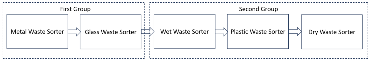
Figure 1. The diagram block of the organic and inorganic waste sorting system
