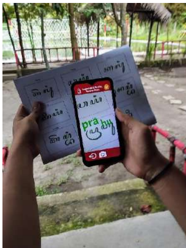
Fig. 5. Example of JawaLens work: all Latin script with green color are augmented on the top of each Javanese script.
