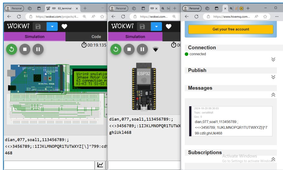
Figure 5. It Can Be Seen That the Connection Data Created on the Project Board Can Be Forwarded to the Hive-MQ Websocket With the Help of the ESP32 Component and the MQTT Protocol
