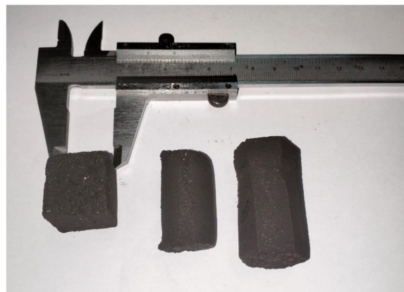
Fig. 1 The cube, tube, and hexagonal briquettes used in this work
