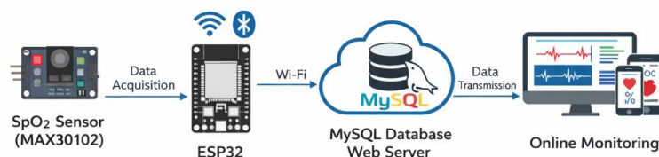
Gambar 1. System architecture of the smart patient bed for SpO 2 and heart rate monitoring.
