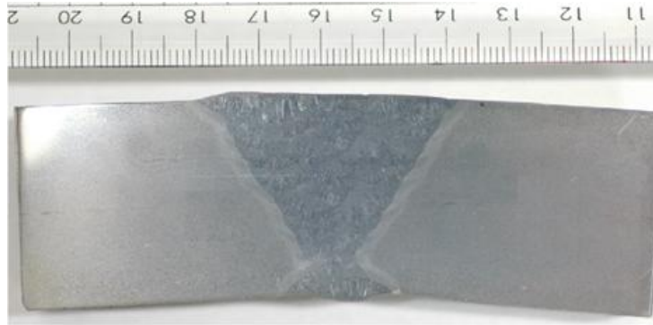
Figure 2. Welded plate of Gr-91.
